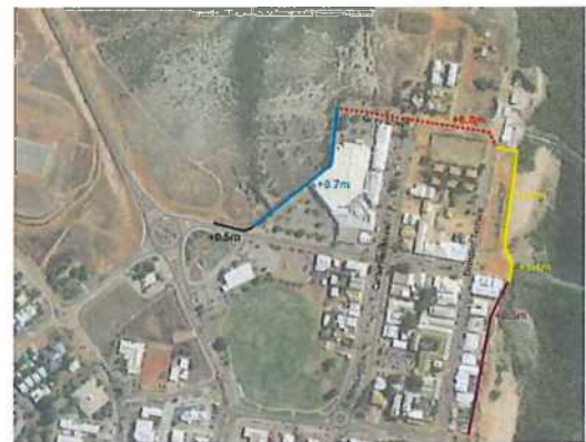
Figure 6.19: Chinatown Inundation Protection Option 1 – required height to raise current peninsula foreshore elements to meet 6.4m AHD.
