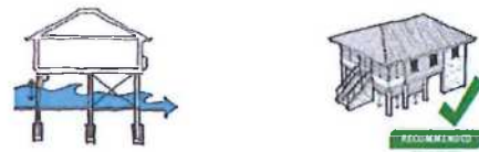
Figure 6.21: Design considerations for buildings in flood prone areas (Queensland Reconstruction Authority)
