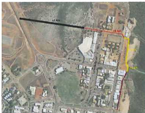
Figure 6.20: Chinatown Inundation Protection Option 2 – Indication of Gray Street extension and required height to raise current peninsula foreshore elements to meet 6.4m AHD.
