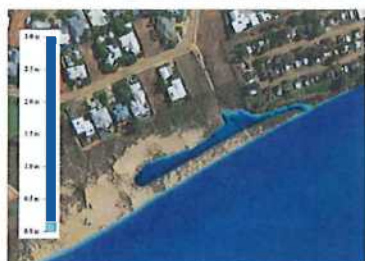
Figure 6.11: Low Point in dune adjacent Demco Drive showing potential inundation in the ARI100yr water level ('bathtub' mapping approach based on LIDAR).
